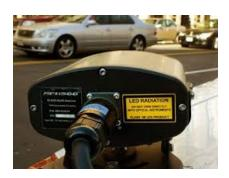
Automatic license plate reader (ALPR): High-speed cameras mounted on poles & patrol cars that record every passing vehicle's license plate, along with time, date and location
